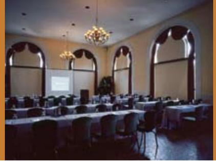
Because it is a blackout fabric, no light can pass through. To ensure that no light at all enters the room when the shades are down, the fabric runs between side channels and the exposed, extruded-aluminum hembar comes to rest behind a sill angle. The rollers themselves are housed within a fascia with a top-back cover that is mounted on the mullion between the window and the windowed arch above it.
