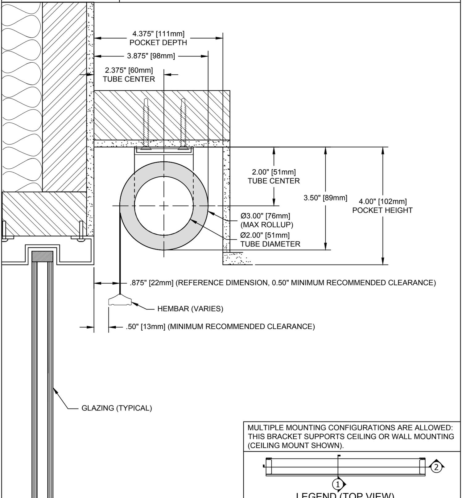
MULTIPLE MOUNTING CONFIGURATIONS ARE ALLOWED: THIS BRACKET SUPPORTS CEILING OR WALL MOUNTING (CEILING MOUNT SHOWN).
