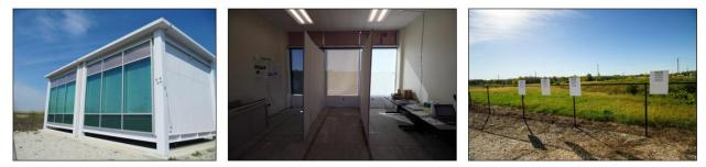
Figure 1: Exterior view of test offices (left), interior partitioning (middle) and Landolt C boards installed outside (right)
