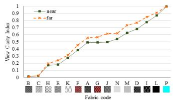
Figure 4: The effect of viewing distance from the window on view clarity score for all fabrics.
