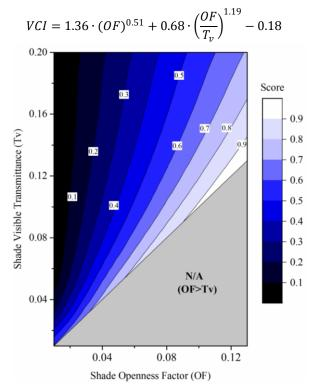
Figure 5: View Clarity Index for various fabric OF and Tv.
