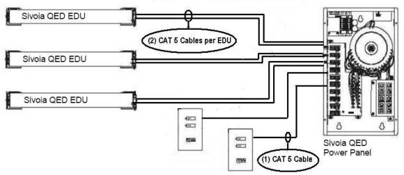
Since CAT 5 is only #24 AWG, the current-carrying capacity is greatly reduced. As a result, when using CAT 5, there must be **two** CAT 5 cables per EDU – one for communications, and one for power. In addition, when using CAT 5, the Sivoia QED communications link must be **home-run** to a SVQ-10-PNL (no daisy-chaining)
