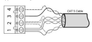
In order to provide the current carrying capability required by Sivoia QED, Common and 12V in the communications link, and the AC power wires **must be tripled-up**. Even with tripling-up these conductors, the maximum wire lengths are reduced.
