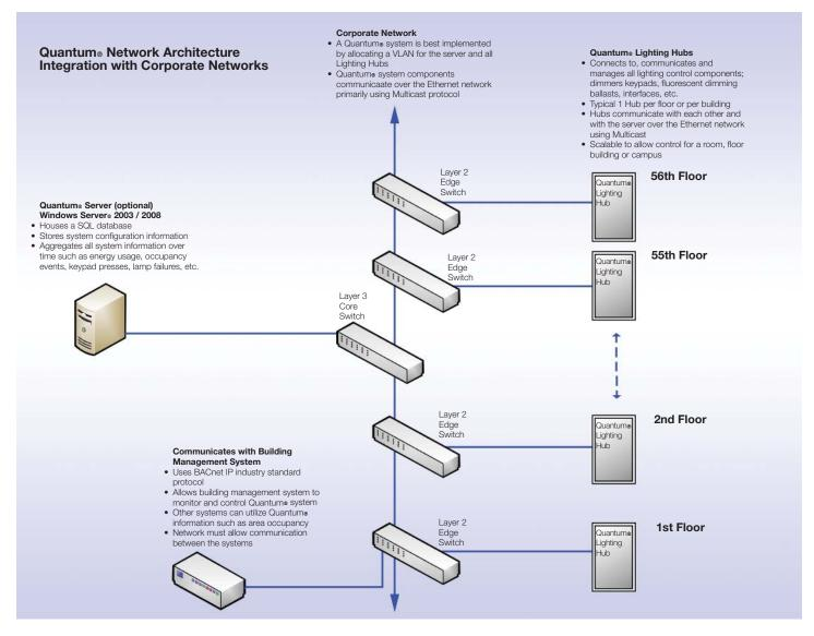
Note: The Quantum<sub>®</sub> server has no BACnet capabilities and thus has nothing to do with the BACnet connection. The BACnet stack exists in the embedded lighting control processors, and thus BACnet connectivity does not require a server running 24/7. Also, connecting to the server directly will NOT provide any BACnet information; the BMS connection must be made to the network on which the Quantum<sub>®</sub> lighting processors reside.
