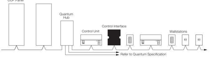
GRX-CBL-46L IEC PELV/NEC® Class 2 wiring cable is available from Lutron and contains: Two 12 AWG (2.5 mm²) conductors for control power.
