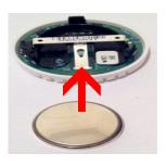
Continue to hold both buttons while sliding the battery back into place. After inserting the battery, continue holding both buttons for about 6 seconds until the LED flashes rapidly.
