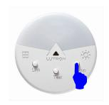
3. Press the Setup button to try the next RF channel (15 total). Press the Test button to repeat the current channel.
