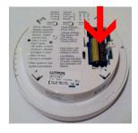
Continue to hold all three buttons while pushing the battery back into place. After inserting the battery, continue holding the three buttons for about 3 seconds until the dome LED flashes rapidly.
