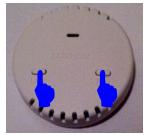
1. Remove the battery from the sensor and hold in the Test and Link buttons.
