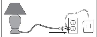
NOTE: This is a POLARIZED cord. It has a polarized plug (one blade is wider than the other) and outlet (one slot is wider than the other).
