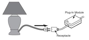
**4.** Insert the Plug-In Module plug into any standard wall outlet.
