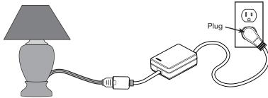
5. Turn the power switch on the load to the full ON position.
