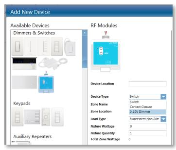
On the left side of the screen the model number will change to LMJ-5T-DV-B. Add the **Device Location**, **Zone Name**, and **Load Type** and click **Done**. This will add the Infratech heater to the area specified.
