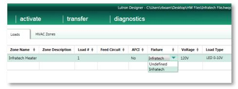
Provide a zone name, zone description, and any other pertinent information. Repeat this process for each Infratech heater that is to be controlled by a neutral wire dimmer driving a GRX-TVI-CPN3876.
