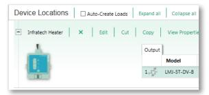
Find the appropriate Infratech heater to assign to the LMJ-5T-DV-B and click **Assign** for that zone.
