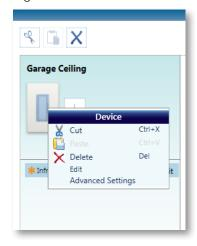
In the *Advanced Settings* screen, fill in the *Low End Trim* and *High End Trim* fields and click *Done*. When using a neutral wire dimmer with GRX-TVI-CPN3876, refer to **Section 6.4** for trim level settings.
