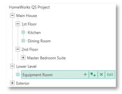
Use the **Equipment** toolbox to add an HWI-PNL-8 dimming panel to the area. If the dimming panel is not currently available in the toolbox, click **Edit Toolbox** and add the dimming panel to the toolbox.
