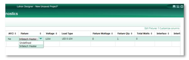
Provide a zone name, zone description, and any other pertinent information. Repeat this process for each Infratech heater that is to be controlled by a LQSE-4T5-120-D zone.
