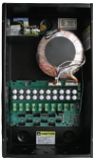
Sivoia QS smart panel power supply (powers up to 10 wired blinds/curtains) QSPS-P2-10-60
