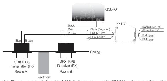
Note: Diagram represents a single partition. A QSE-IO will accommodate up to five GRX-IRPS partition sensors (five partitions). A single PP-DV will power one GRX-IRPS partition sensor.
