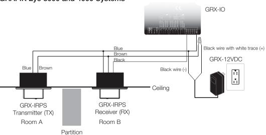
Note: Diagram represents a single partition. A GRX-IO will accommodate up to five GRX-IRPS partition sensors (five partitions). A single GRX-12VDC will power up to eleven GRX-IRPS partition sensors.
