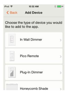
Once the Pico Remote has been chosen, the app will show how to add a Pico Remote to the Smart Bridge. Ensure that the proper Sleeve Button is being pressed and held. For more information on the button mapping of the Sleeve Buttons, based on its orientation on the wall, refer to **Appendix A**.
