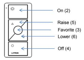
Notice that when the buttons are oriented to the left of the iPad, the mapping is reversed or upside-down. This is important to understand in order to program the appropriate functionality to the correct button in the Lutron programming software.
