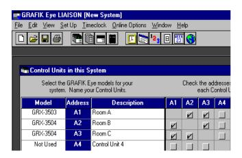
**NOTE:** New scenes can be created based on room configurations. Wall wash zones focused on partitions can become "downlights" or turned off when partitions are removed. Additionally, GRAFIK Eye Control Units could be electronically locked out (i.e., when all partitions are open, Control Units 2 and 3 could be set up in "4S" mode to allow only scene activation from those Control Units).
