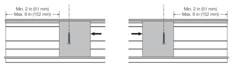
NOTE: If the hole in the Stiffener and the pre-existing mounting screw hole in the Mounting Rail cannot be aligned, it will be necessary to drill a new hole in the Mounting Rail which allows the mounting screw to pass through the Stiffener as noted in step 4.3 below.
