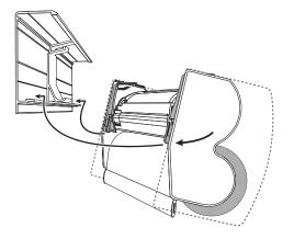
WIDE SHADES WITH CENTER SUPPORT: The Center Support is positioned to cradle the shade's battery holder. On wide shades, the center of the battery holder may sag during installation step a., requiring you to lift it up and into the cradle as you proceed to step b.
