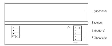
Faceplate is comprised of a top and bottom. The bottom will always be the colour indicated under "faceplate." The top may be the same colour or translucent. Use the chart for faceplates that have the same colour top and bottom. If a translucent lid is chosen, the stripe will automatically be the same colour as the bottom lid.
