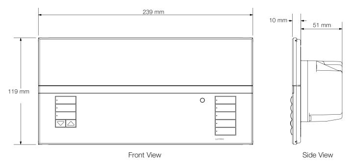
Fits into a 4-gang U.S. backbox, 90.4 mm deep (Lutron P/N 245-254) or 76.2 mm deep (Lutron P/N 241-400)
