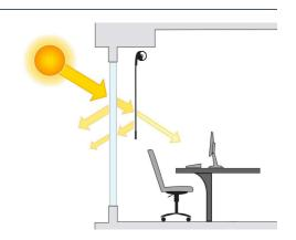
**Solar Reflectance (Rs)** - the solar reflectance of a shade fabric is the percentage of total radiation that is reflected off the exterior face of the fabric. Although the glass may reflect some of the radiation back into the space, shades are able to reflect solar heat back out of the building.
