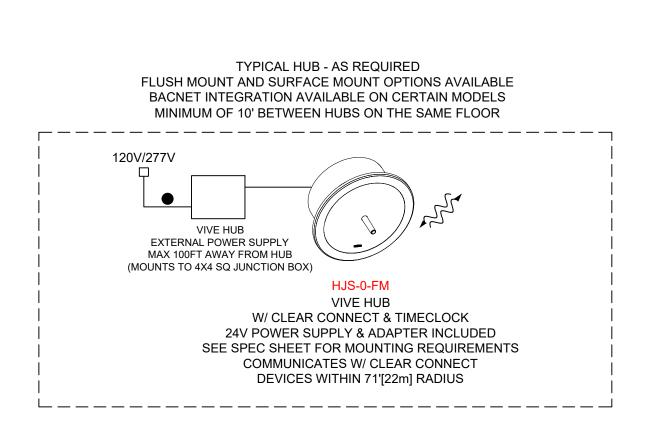
TYPICAL SENSORS & REMOTE CONTROLS CAN BE A MAX OF 30' TO LOAD DEVICES -MAX OF 71' FROM VIVE HUB AND LOCATED ON THE SAME FLOOR
