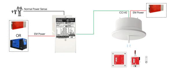
As of April 2022, the Vive Emergency PowPak will no longer carry the UL 924 mark. The Vive Emergency PowPak is still integral to a simple Vive solution for use in emergency lighting systems in accordance with UL 924.
