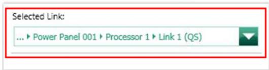
2. Activate the Power Modules on the QS links by either pressing and holding a button on each Power Module, manually entering each Power Module serial number, or scanning each Power Module serial number. The Power Modules must be activated before activating and addressing any EcoSystem drivers/ballasts.
